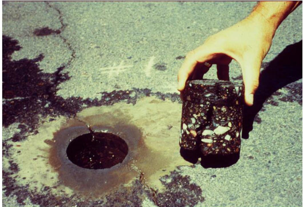
Slight movements associated with old cracks or joints are dissipated by the membrane. More importantly, even if the crack reflects through, the membrane remains intact and continues to *waterproof*.
